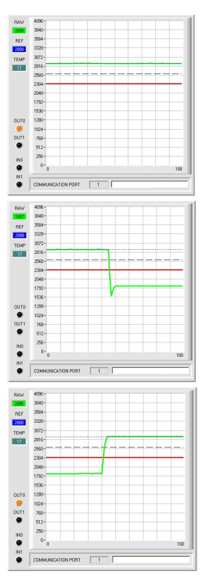
As long as the current measurement value **RAW** (green line) lies above the switching threshold (red line), the output **OUT0** has +24V (signal is OK). This is visualised by the **OUT0** LED.
